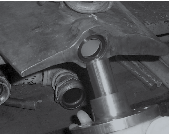
ThorPlas Wicket Gate Bearing with Thorseal
