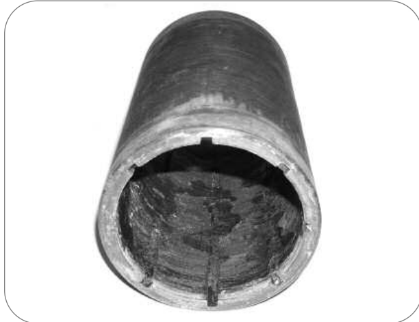
Typical example of a wiped bearing.
