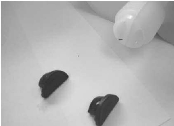
Figure 2: Plugs for TG-75 cartridge.
