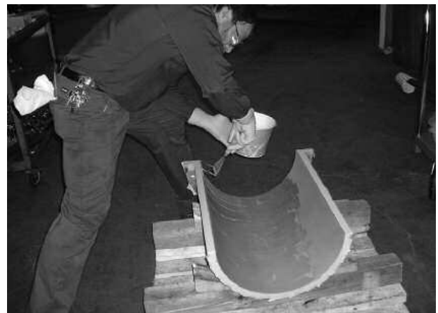
Figure 5: Adhesive applied to split metal housing.
