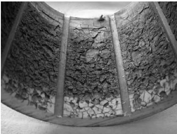
Typical example of bearing with hydrolysis.
