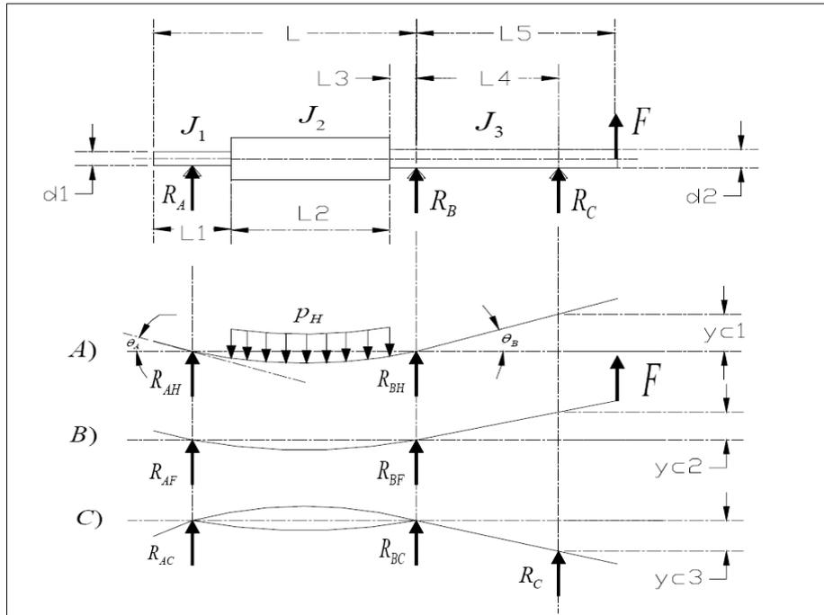
Figure - 3: Loading diagram
