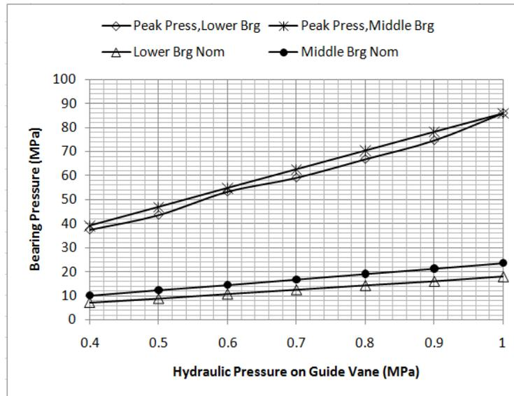
Figure – 5: Peak and Nominal Bearing Pressure (MPa)
