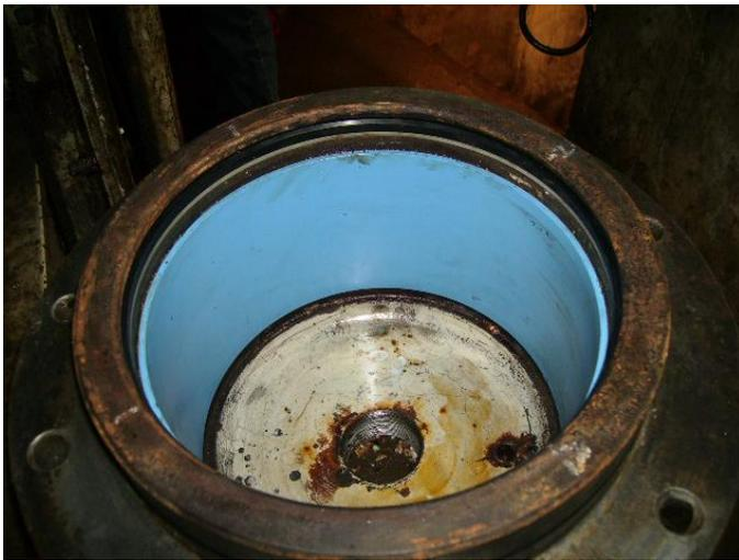
Figure - 6: One Lower Bearing after 8 months operation
