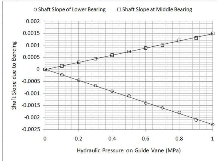
Figure - 4: Shaft Slope for Middle and Lower bearings
