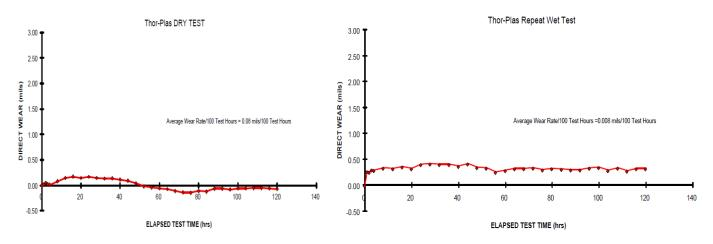
In Fig -2b, after making the initial displacement zero, the calculated wear rate for wet test was actually lower than dry condition. The average adhesive wear during 100 hours was 0.08 mils (1 mil = 0.001 inch)
