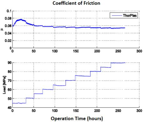
Fig – 4: Coefficient of Friction reduces with time and increased pressure
