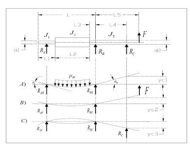
Fig - 10: Loading diagram of a typical wicket gate shaft [4]
