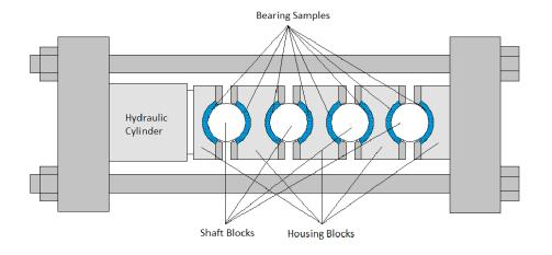
Fig – 6: Schematic of Creep Test Rig
