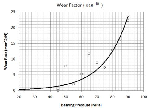
Fig – 5: Wear factor as function of bearing pressure
