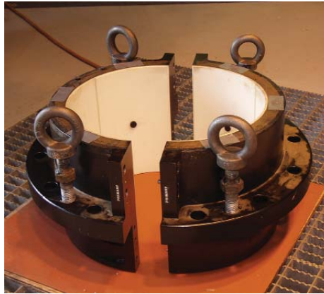
Thordon SXL Main Guide Bearing ready for installation at Star Lake
