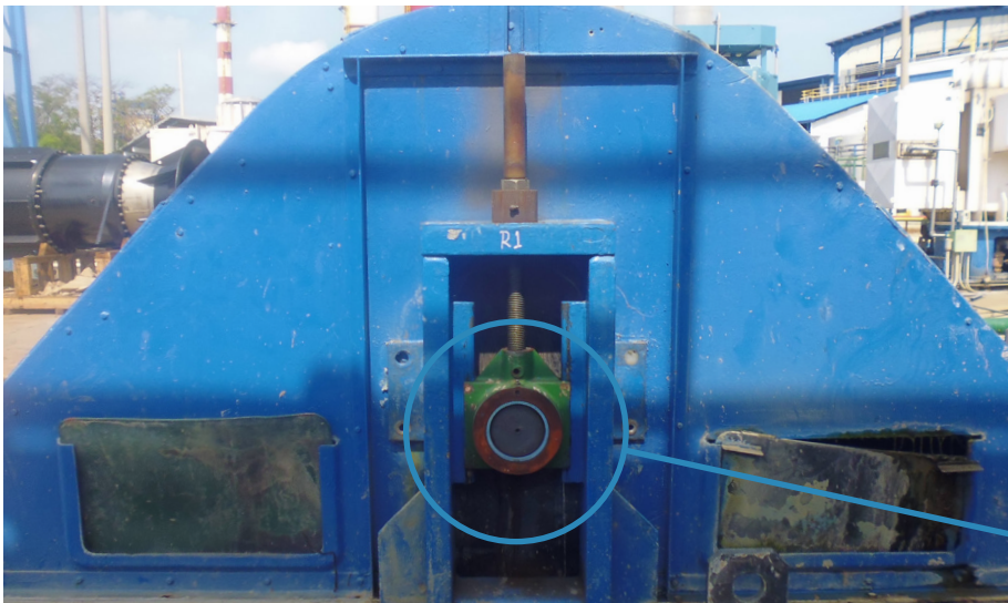
ThorPlas-Blue bearing after installation
