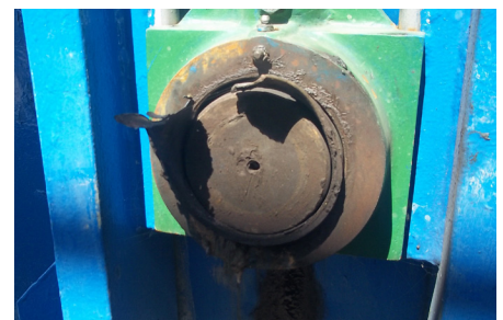
Initial situation of bronze bearing after 3 months of operation
