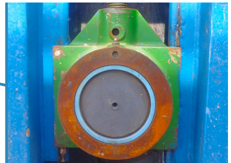
ThorPlas-Blue bearing installed
